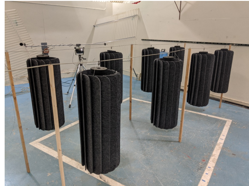
Figure 1 – Specimen mounted in test chamber
