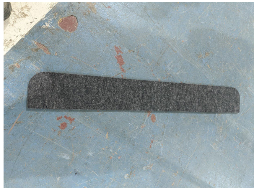
Figure 4 – Individual specimen fin prior to installation to hub
