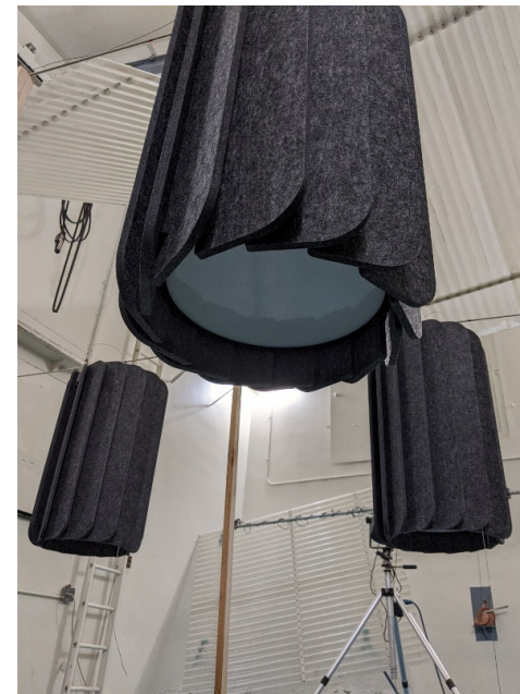
Figure 2 – Acrylic lens at underside of specimen, orientation of felt fins
