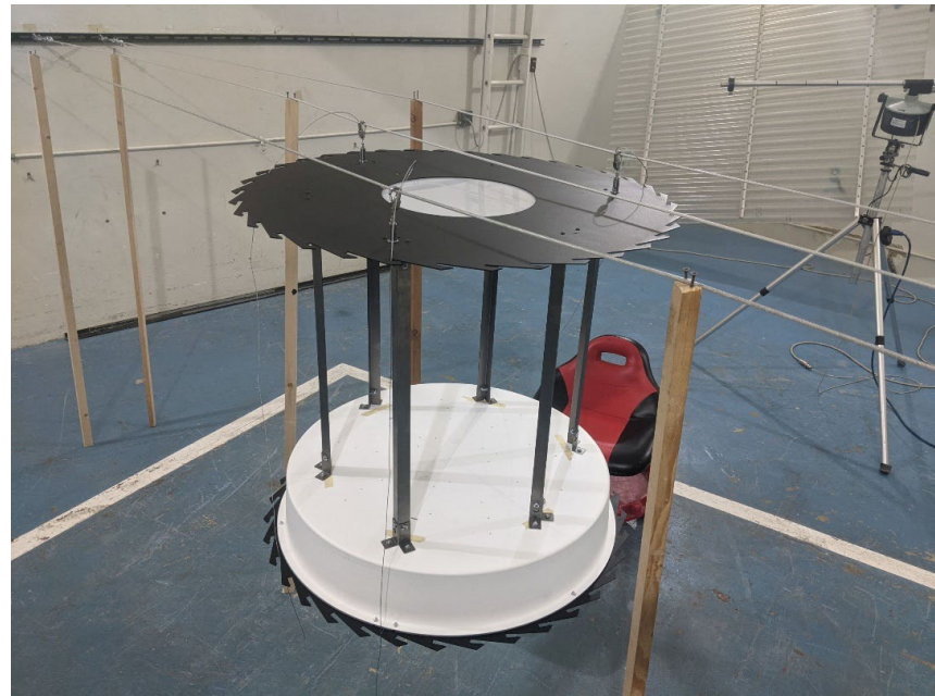
Figure 3 – Specimen top and bottom hubs connected by “V” columns
