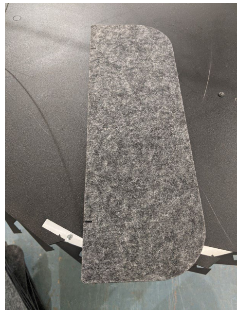
Figure 4 – Individual specimen fin prior to installation to hub
